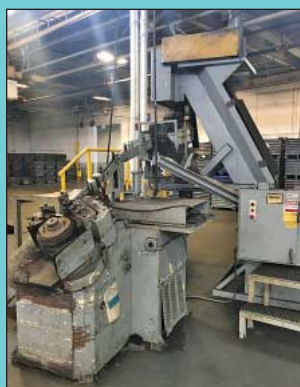
Pruetton Model 200SV Thread Roller Set up as Stud Roller w/ Vibratory Bowl
